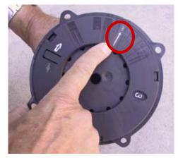
The arrow with the no. 3 marks the direction in which your slope shows.
